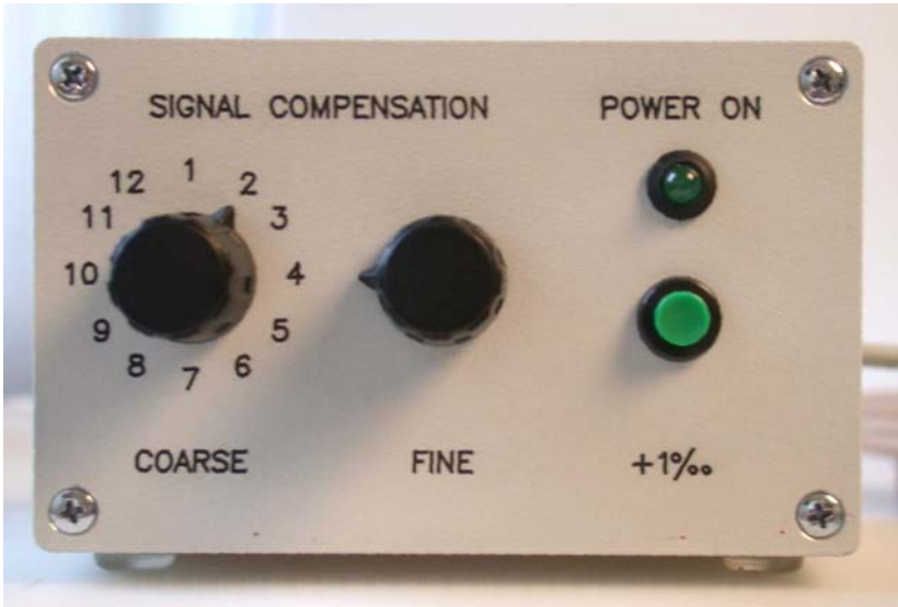
Fig. 2: Front view of LED-Driver and Compensation Unit ED-P700DW-T
